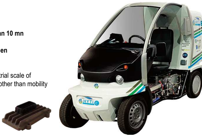
RMS tank management system (SOC status, thermal management, flow management, ...)
